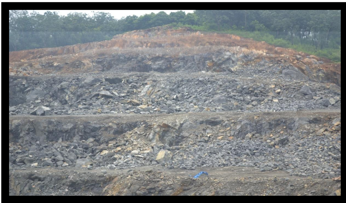
Minerals explored with bench system of 5 m width and height
