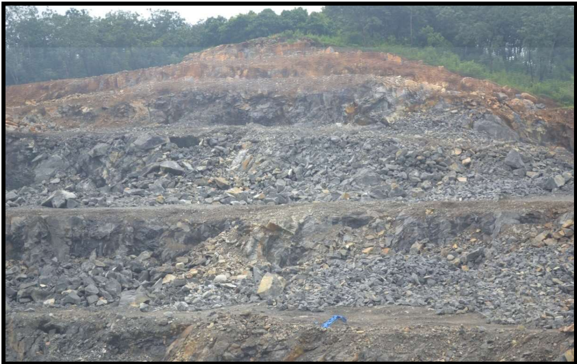
Minerals explored with bench system of 5 m width and height
