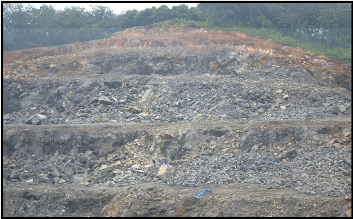
Minerals explored with bench system of 5 m width and height
